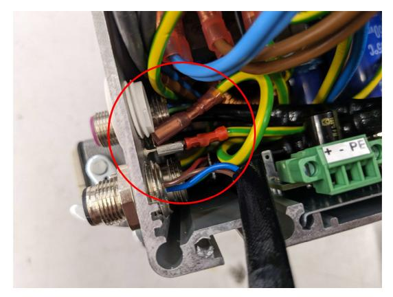
9. Connect IN and OUT lines to the bus board.
