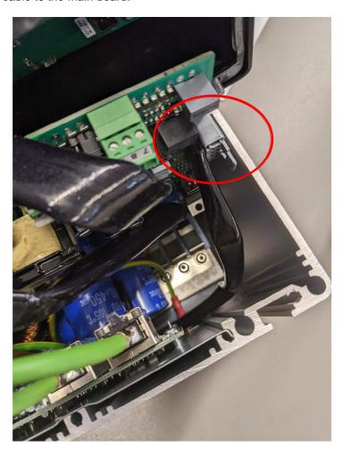
8. Connect the PE cable from the device to the PE cable of the bus board and connect them together to the PE connector on the housing.
