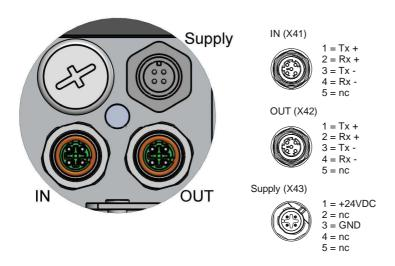
The interface enables communication with the frequency converter, using 4 data words (i.e. 16 Bits). The four 16 Bit words are transmitted and acknowledged every bus cycle.
