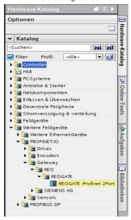
In the following example, a REO device has been linked to the control PLC. Address and name were given by TIA, but can also be changed afterwards.
