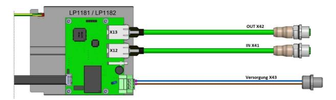
10. Connect the 24 V supply to the terminal (+ - PE) of the bus board and screw hand-tight to the PCB.
